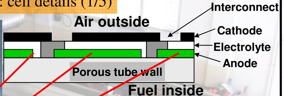
Section through one wall of tube
