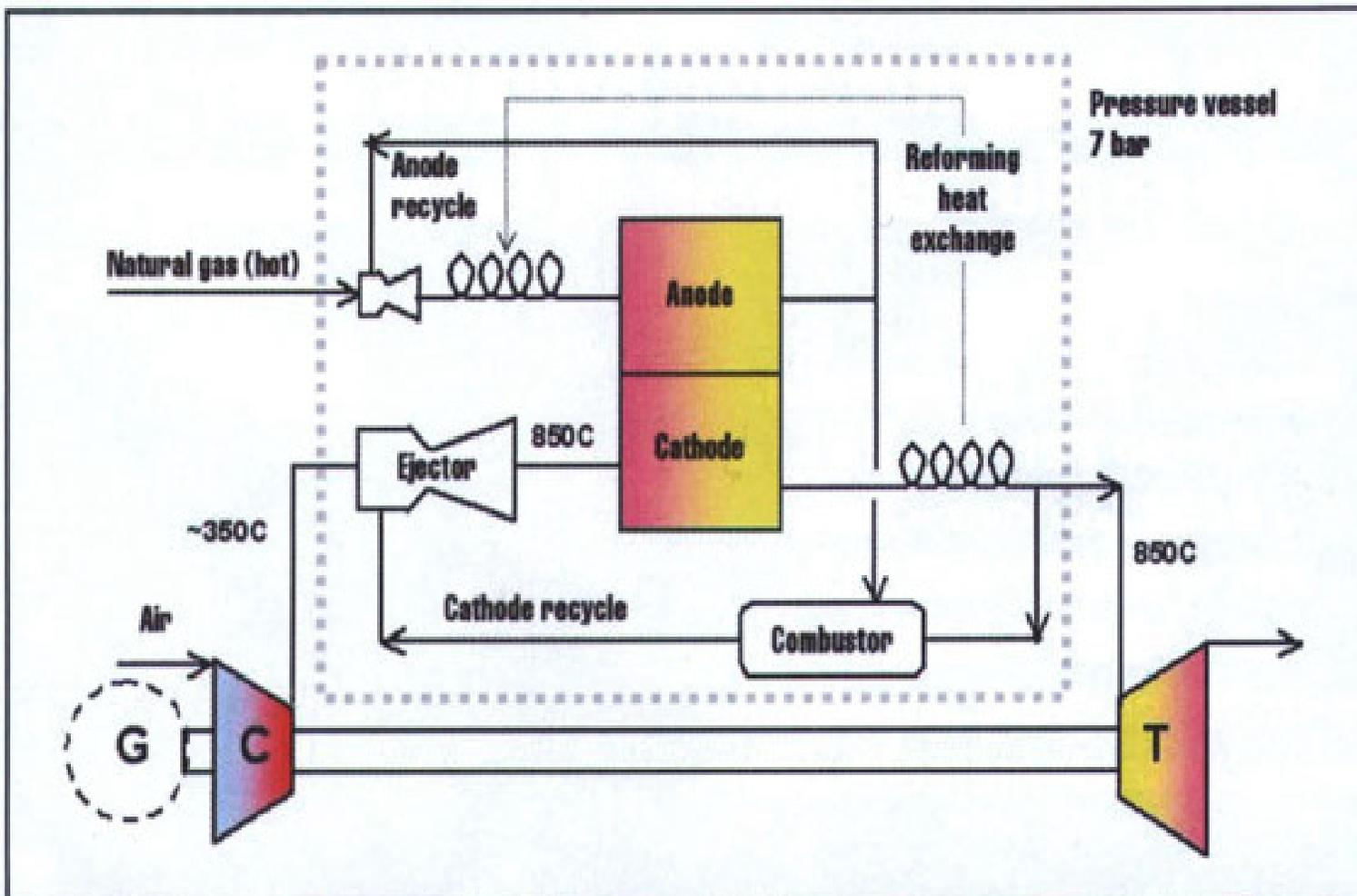
Rolls-Royce's novel solution: the heat-exchanger-less SOFC hybrid cycle. The system is pressurised to 7 bar
